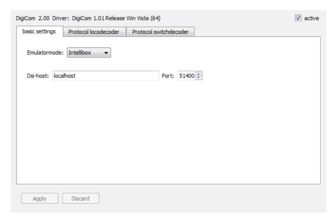
**Emulator mode:** DigiCom simulates an Intellibox or a Märklin-Interface 6051. Please enter which command station your control program supports. If both will be supported you should prefer the Intellibox.
