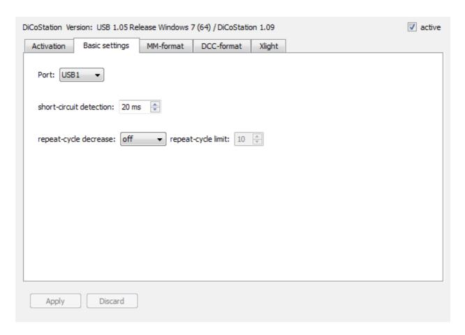
**Port:** Each DiCoStation will create an own ongoing port number by connection to the USB. This procedure will assure that the correct DiCoStation will be contacted if temporary not all DiCoStation are connected. If only one DiCoStation is connected this station has the number USB1.
