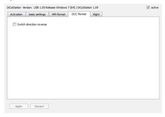
Switch direction reversing: Reversing the switch direction of all magnetic accessories.
