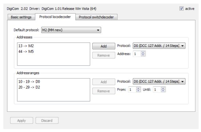
**Default protocol:** Here you can enter which protocol shall be used if no single address or address range has been indicated or applied.
