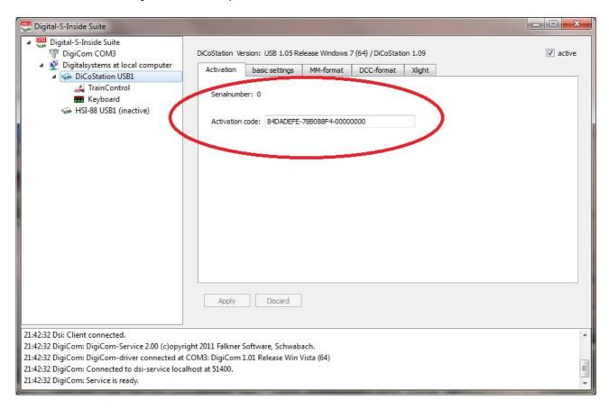
Without a valid activation code the operation of the DiCoStation will be running in demomode.
