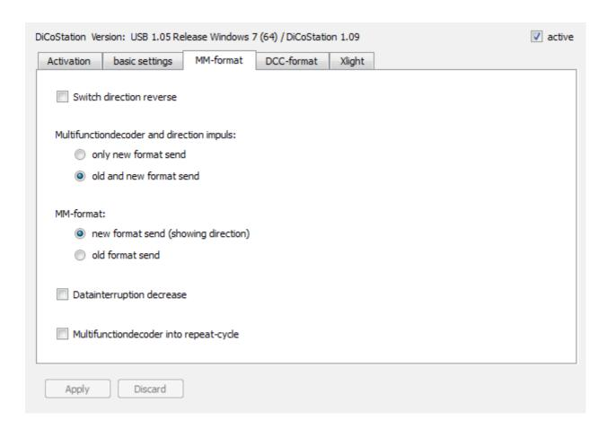
**Switching direction reversing:** Reverse the switching direction of all magnetic accessories.
