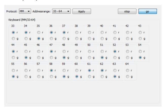
For testing please select the protocol and the address section of the switch decoder and click onto "apply". Now switch buttons for switching will be indicated.
