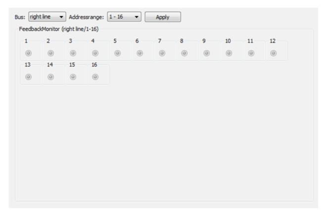
Select the bus and the address range of the feedback decoder and click onto "apply". The status of the feedback contacts will be indicated.
