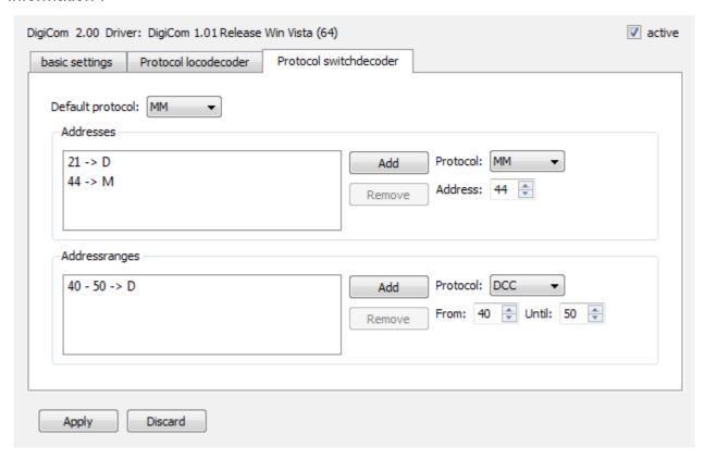
**Default protocol:** Here you can enter which protocol shall be used if no single address or address range has been indicated or responded.
