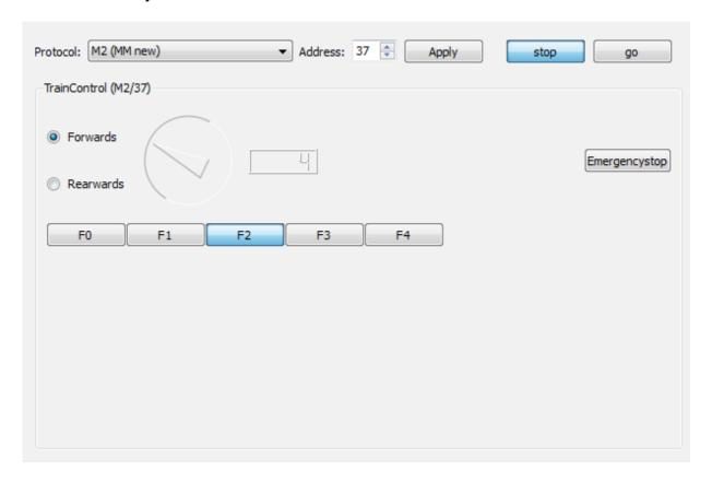
Select the protocol and the address of a Loc-Decoder then click onto "apply". Now will be a speed regulator and function keys indicated corresponding to the selected protocol.
