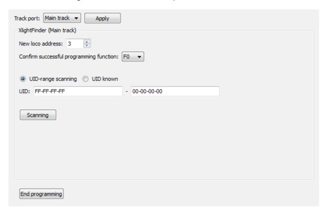
To assign an address to a locomotive select at first the track connection which is connected to the track where the loc is located. The DiCoStation contains no programming-track therefore the main track has to be used. Activate now the button "Apply". Enter now the address for the loc. Select the switch-function (F0 – F15) for the confirmation of the successful programming.
